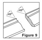
To span longer lengths, you may have to splice your crowns. Set your mouldings in a mitre box or compound mitre saw as described in previous section. Mitre the joining ends at 45° angles from front to back. One piece will overlap the other in a scarf joint. (Fig.9), creating a vertical face seam in the finished installation.
