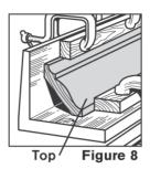
As described, crowns do not lie flush against the wall. Cutting correct 45° mitres is critical. Clamp two blocks of wood to the mitre box to hold the moulding in place at the angle at which it will be installed. Once blocks are in place, insert moulding prior to cutting, face out and upside down (Fig.8). Then cut
